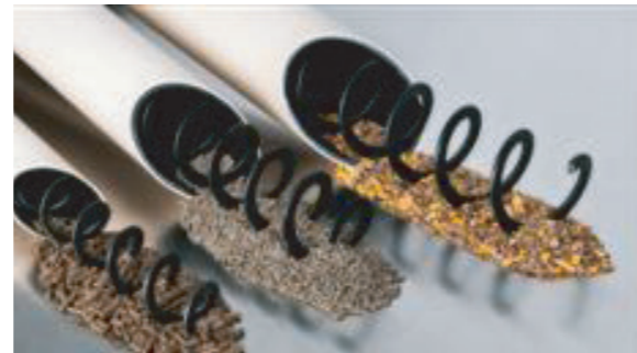
Conveyor spirals and augers
